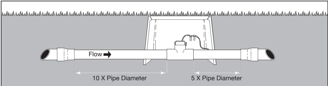
**Note:** For 1.5" and larger flow sensors, install according to the flow direction shown by the arrow on the tee. For 1.0" and smaller flow sensors, installation is not dependent on flow direction.
