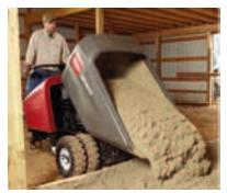
**Powerful** Easily transport up to 2,500 lbs. loads and discharge smoothly with fully hydraulic dump system.
