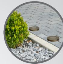
Robust, discrete and versatile describes the Solstice design and function. A powerful in-ground well light, the Solstice is drive-over rated. The Solstice can cast an ample beam spread against any landscape element. The internal stainless steel gimble ring holds the secondary cast brass and glass-filled nylon body in place while allowing vertical and horizontal adjustments within the composite body.
