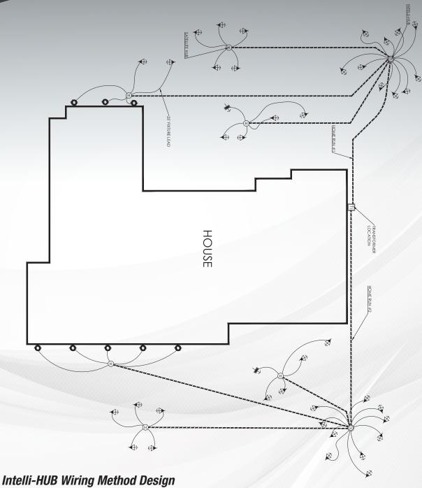
Shown here is an actual Intelli-HUB wiring design. As you can see, the Intelli-HUB wiring method not only reduces the number of connections in the field, it is the safest way to install low voltage lighting. By fusing HUBs in the field, total system failures are greatly reduced. Allowing you to enjoy your system for years without worry of a short or a redesign years down the road. A few advantages of the HUB wiring method:
