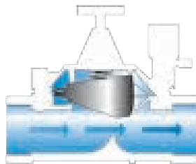
The UltraFlow Series straight-through flow path
