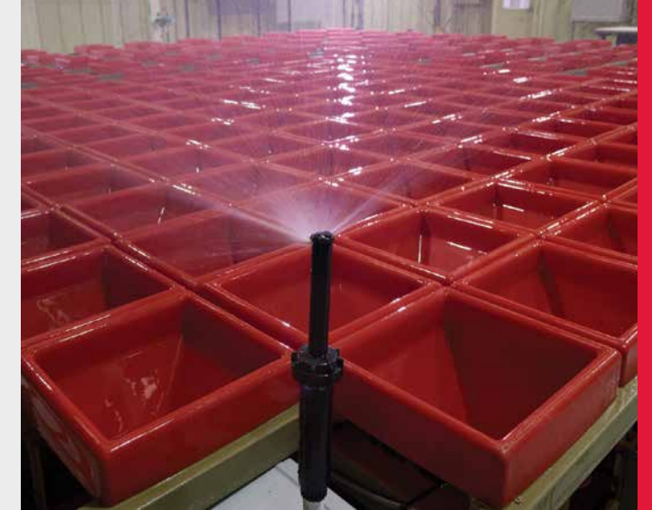
Laboratory and third party independent field testing show efficiency to be 15-20% higher than competitive nozzles at 4,6m or less.
