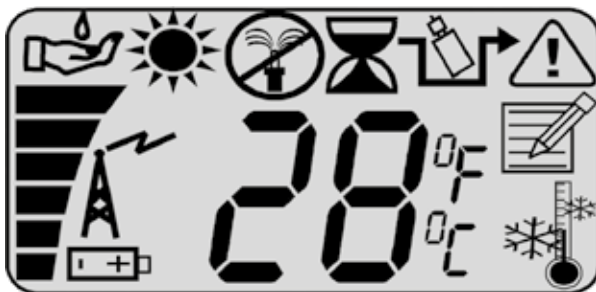
First LCD In A Wireless Rainsensor Provides informative system feedback including outside temperature, and transmitter signal strength and battery life.
