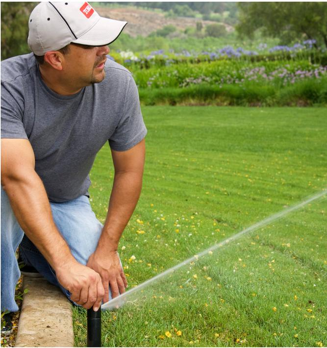
Rotating nozzles deliver multiple streams of water with different distances in each stream. Rotating nozzles have a reputation for applying the water at a rate that makes it easier for the ground to absorb the moisture, and as a result, are often recommended for slopes. It's important to note that rotors also apply water slowly, making them a great choice for tight soils and slopes.
