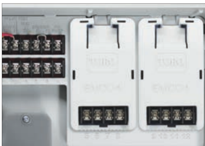
12-station configuration with two 4-station modules (EMOD-4)
