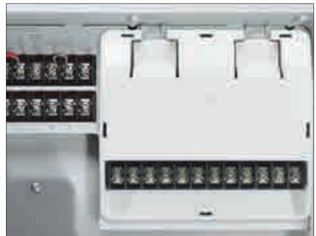
16-station configuration with one 12-station module (EMOD-12)
