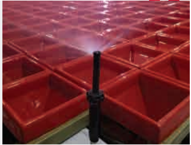
Laboratory and third party independent field testing show efficiency to be 15-20% higher than competitive nozzles at 15 feet or less.
