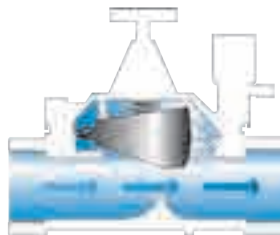
The UltraFlow Series straight-through flow path
