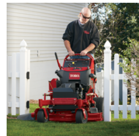
ULTRA-COMPACT FOOTPRINT Ideal for smaller residential properties or areas with gates and tight spaces, available in 91cm and 102cm models.
