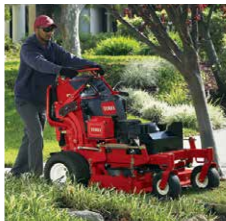
2-IN-1 VERSATILITY Toro's fold-up operator platform allows conversion of the GrandStand to a walk-behind. Just lower it back down to ride – no need to switch mowers.
