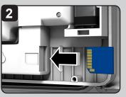
Insert SD card into the Smart Connect's SD card slot.
