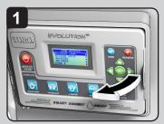
The controller must be powered on. Open the EVOLUTION controller's front panel.
