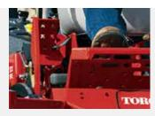
DECK LIFT ASSIST Standard deck lift assist foot pedal allows operator to adjust the deck height quickly and easily.
