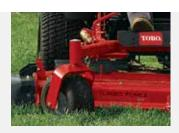
PRO RESULTS EVERY TIME TURBO FORCE® 5.5" deep cutting decks feature 18,500+ ft./min. blade tip speed and nearly 1/4" thick heat-treated steel blades.
