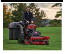
The patent-pending side-mounted Soft Twin Bagger has a large 10 cu. ft. (8 bushel) (0.28 m³) capacity and the vertically-mounted blower allows for excellent maneuverability in tight spaces and maximum visibility.
