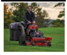
The patent-pending side-mounted Soft Twin Bagger has a large 10 cu. ft. (8 bushel) (0.28 m3) capacity and the vertically-mounted blower allows for excellent maneuverability in tight spaces and maximum visibility.
