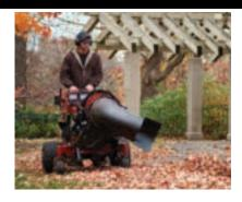
The Pro Force Blower has a 360° nozzle rotation and utilizes the MULTI FORCE 26.5 hp Kohler® Command Pro™ EFI engine to deliver tremendous air power for fast removal of grass clippings, leaves, or other debris.
