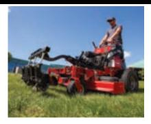
Puncture up to six holes per square foot with the 38" wide aerator. Tines pierce deep into the soil, hooking and lifting loose plugs of dirt that disperse quickly, spreading nutrients over the surface.
