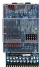
**KIT D'ENTRÉE DE CAPTEUR POUR LYNX® SMART SATELLITE**
