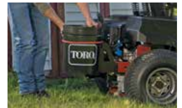
BUCKET MOUNT KITS Part #136-7494 (TimeCutter HD) Part #133-2533 (Toro 5-Gallon Bucket)
