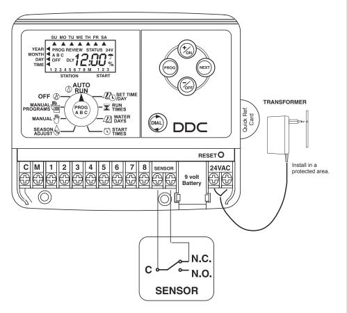
To connect a rain sensor, remove the jumper wire from the sensor terminal and connect one wire of the Toro RainSensor<sup>™</sup> to the C-common terminal and the other wire to the N.C. (normally closed) terminal. As soon as the Toro RainSensor<sup>™</sup> contacts change from the N.C. position to the N.O. (normally open) position, irrigation will be suspended. Irrigation will resume as soon as the Toro RainSensor<sup>™</sup> dries and its contacts return to the N.C. position.
