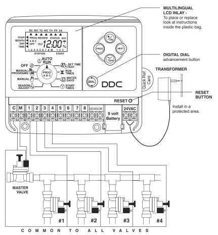
Remove the lower cover of the DDC controller. Place the unit on the wall using the top screw slot. Level the controller, then insert screws into the two lower screws holes under the terminal block. Connect the solenoid wires to the terminal block. Connect one wire from the solenoid to its respective station number on the terminal block and the other wire to the C-common terminal. Finally, connect the transformer wires to the 24 VAC terminal. Next install the battery.
