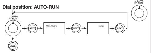
The AUTO-RUN position is used to provide information regarding the controller's operation as well as for reviewing all data stored in the irrigation programs. The following is a list of information you can observe on the display:
