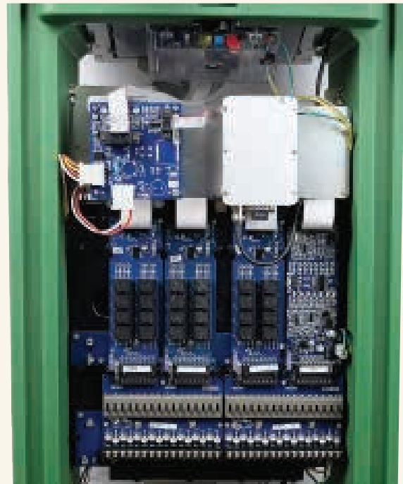
Network VP Satellite with Vertical Power Distribution Board and Digital Radio Kit (RADIOKIT-V-G)
