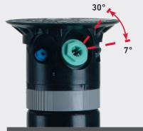
Trajectory – 24 Positions From 7° - 30° in 1° increments put water where you want it. Adjust from the top of the sprinkler in seconds, wet or dry. This flexibility lets you tackle every obstacle on the course; wind, trees, bunkers, mounds and more.
