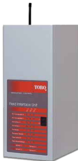
Field Interface Unit The LYNX computer is attached to a Field Interface Unit (FIU) which sends commands to the SmartHubs throughout the golf course. There are two ways for the FIU to communicate with SmartHubs: by Wireline or by radio.
