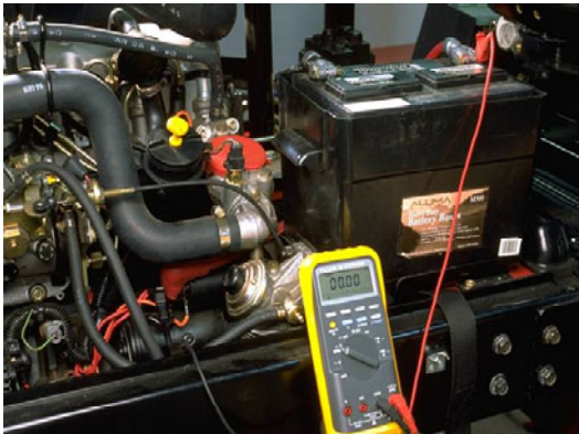
Voltage Drop Testing (Feed Side)
