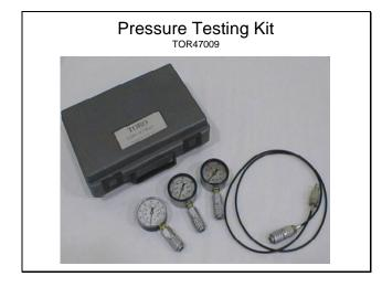
Hydraulic test equipment allows you to observe the amount of oil pressure and oil flow in a circuit under various conditions.
