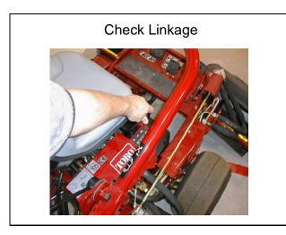
Check the control linkage for improper adjustment, binding or broken parts.
