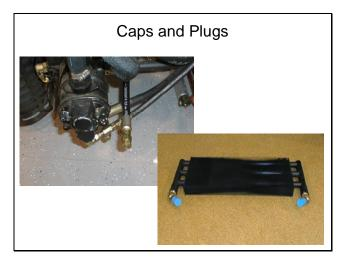
Put caps or plugs on any hydraulic lines left open or exposed during testing or removal of components.
