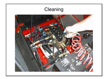
Thoroughly clean the machine before disconnecting or disassembling any hydraulic components. Always keep in mind the need for cleanliness when working on hydraulic equipment.
