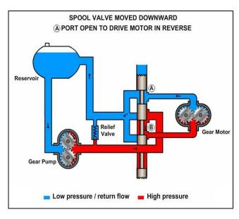
This illustration shows the basic circuit and components necessary to drive the cutting unit reels. With the spool in the upward position, the oil flow is directed through the spool valve to the lower port driving the motor in the forward direction.
