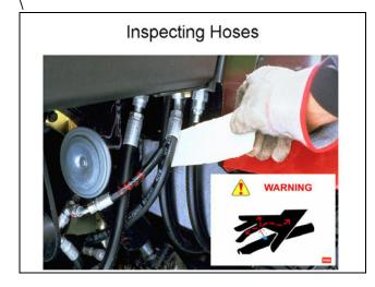
Before disconnecting or performing any work on a hydraulic system, all pressure in the system must be relieved by stopping the engine and lowering or supporting the implement.
