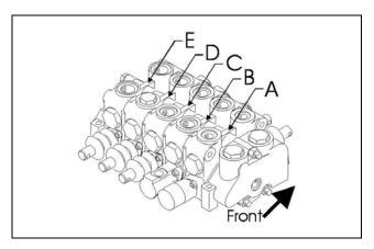
This is that same spool valve, assembled with multiple sections to make a valve bank or assembly. This example is from a Greensmaster riding mower. In this example the valve bank would control all of the hydraulic functions on the machine and would be actuated by foot or hand operated levers.
