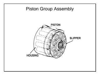
The pump consists of the following components:
