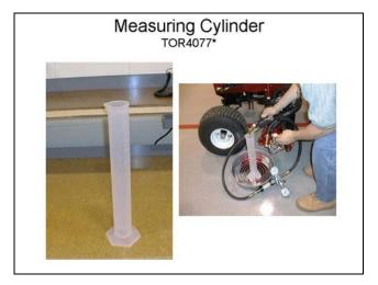
This measuring cylinder is used to measure flow on very low flow circuits. An example is measuring the flow from the case drain line of a hydraulic motor to test for motor efficiency.
