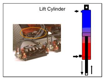
The flow diagram in the previous two illustrations shows the piston (barrel) end of the cylinder being pressurized to lift the load. Some lift circuits on Toro equipment pressurize the rod (ram) end of the cylinder to lift the load (e.g. Reelmaster 5000 series).
