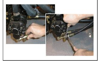
Install fittings finger tight, far enough to insure that they are not cross-threaded, before tightening them with a wrench.
