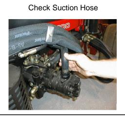
All hydraulic test should be made with the hydraulic system at normal operating temperature. Check for soft or collapsed suction hose.
