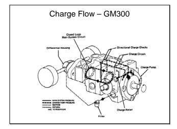
Here is a view of the closed loop main circuit and charge circuit within the inline hydrostatic transmission from a Groundsmaster 300 Series.
