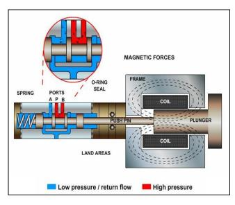
The electric solenoid valve operates by supplying electrical current to a coil magnet, the magnetic field moves a valve spool and this directs the oil. The thing to remember is that the only difference between a hydraulic\electric valve, and a manually actuated hydraulic valve is the way that the spool is moved.
