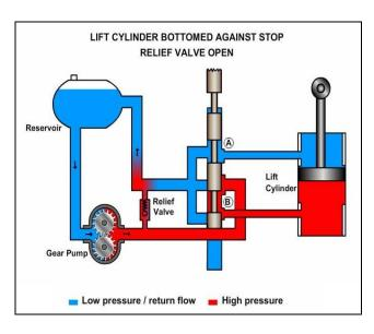
Since the fluid from a positive displacement pump must flow continuously whenever the pump is running, it must have some where to go if not being used by the actuators. If the load on the cylinder becomes too great or if the ram bottoms out, the flow from the pump will be directed past the relief valve returning to the reservoir.
