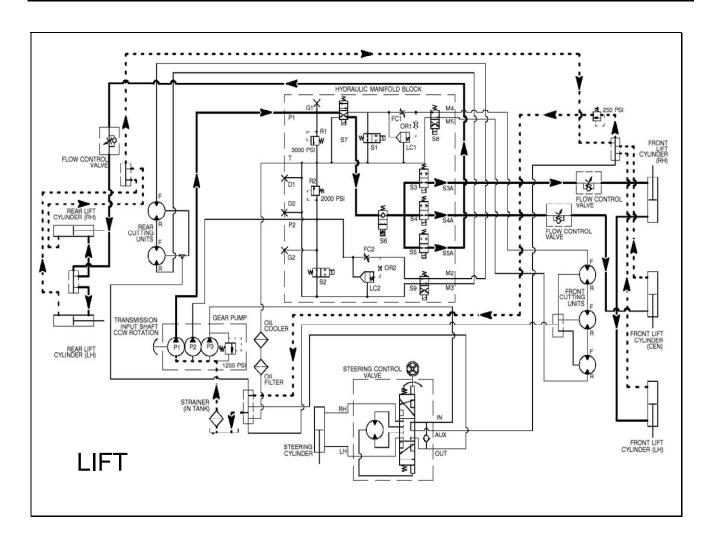
The key to understanding complex schematics is to break them down into their individual circuits. If you are troubleshooting a lift/lower problem, you don't need to be looking at the cutting drive or steering circuits.
