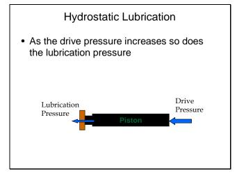
One piston is shown here illustrate the principle that the drive pressure increases so does the lubrication pressure for the piston slipper and swash plate surface.
