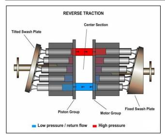
When the operator needs to change directions the traction pedal is moved back to the neutral position and than moved to the reverse position. In the reverse position the swash plate moves in the opposite direction as it did in the forward direction. In this position the oil is pumped to the opposite side of the motor and the unit moves in reverse.
