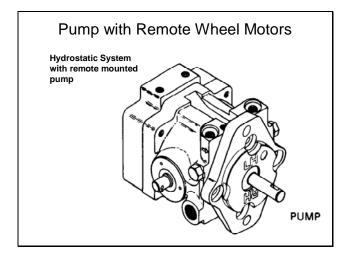
The first type is a hydrostatic system which consists of a hydrostatic pump with a remotely mounted motors. In this type of hydrostatic system the hydrostatic pump is mounted by, and driven by, the units engine. The pump is connected to the drive motor by hoses or steel lines. These motors can be mounted directly to the wheels or to a drive axle.
