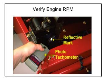
The engine must be in good operating condition. Always use a tachometer when doing a hydraulic test. ENGINE SPEED WILL AFFECT THE ACCURACY OF THE TESTER READINGS.
