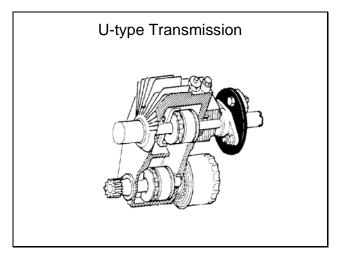
A similar version is the U-type transmission. In this type of system the pump and motor are constructed as a common component with the pump usually located above the motor.
