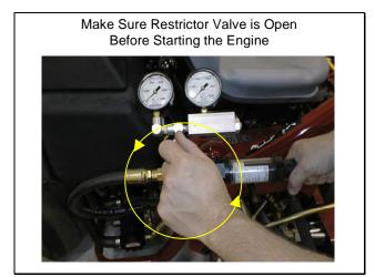
To minimize the possibility of damaging the components, completely open the load valve by turning it counter clockwise (tester with pressure and flow capabilities).
