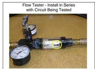
To prevent damage to the tester or components, the inlet and outlet hoses must be properly connected and not reversed (tester with pressure and flow capabilities).
