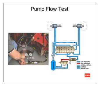
This is an example of a pump flow test. This test is also known as a pump efficiency test.
