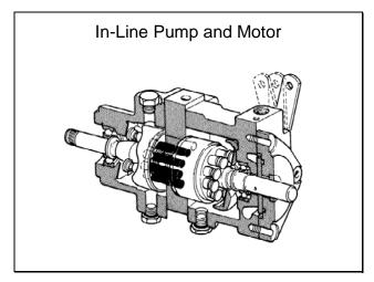
A different type of hydrostatic drive system is an inline pump and motor system. In this system the motor and pump are constructed as a single unit, this eliminates the necessity of high pressure drive lines between the pump and the motor. This unit is normally mounted to a drive axle or transaxle.
