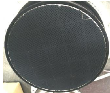
Figure 2 - This DPF filter is clogged with PM due to prolonged low-load engine operation, extended low rpm idle time, or lack of maintenance.
