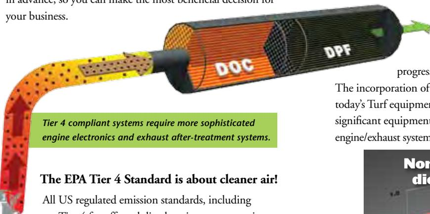
Tier 4 compliant systems require more sophisticated engine electronics and exhaust after-treatment systems.
