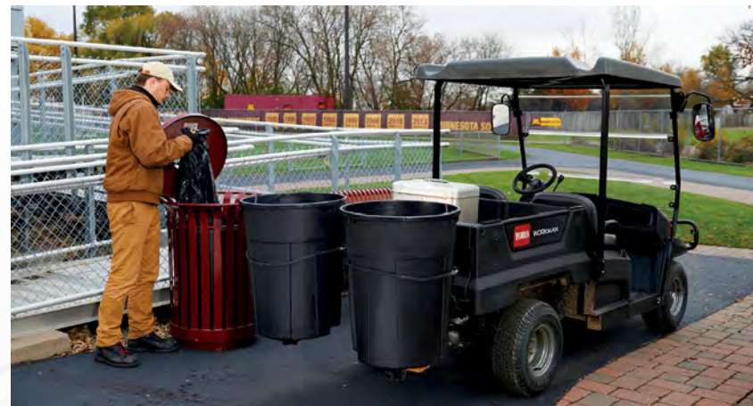
Dual garbage/recycling container mount attachment allows customers to set up a vehicle for morning trash collection, and quickly remove for normal run-around vehicle needs.
