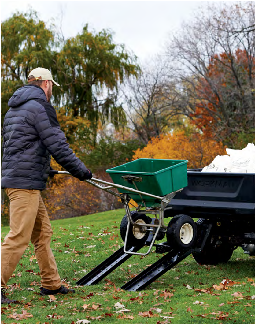
A universal walk spreader mount with self-storing ramps eliminates lifting the spreader in and out of the back of the vehicle. Simply push it up the ramp, store and go.
