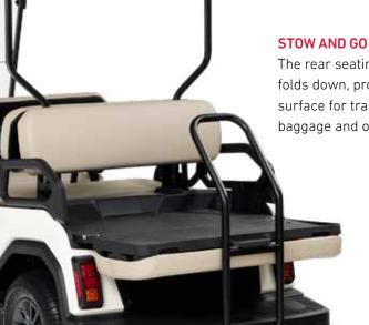
The rear seating section folds down, providing a flat surface for transporting baggage and other cargo.
