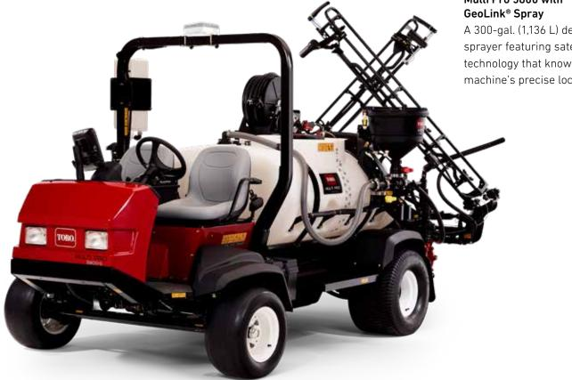
Multi Pro 5800 with A 300-gal. (1,136 L) dedicated sprayer featuring satellite-based technology that knows the machine's precise location.
