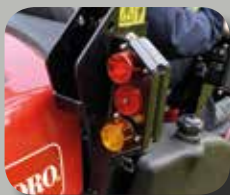
LED Lighting kit with brake lights
