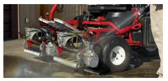
Sealed electrical components for worry-free wash down.
