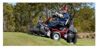
**More power for higher performance.** A 21hp Vanguard<sup>®</sup> Twin gasoline engine and a 23.5 hp Kubota<sup>®</sup> diesel engine, both in hybrid and hydraulic options, have ample power for any application.
