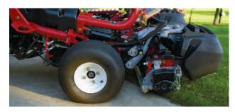
**Stay ahead of the game.** A generous 5" (12.7 cm) ground clearance protects cutting units in transport and when climbing curbs. Fast 10 mph (16 km/h) transport speed also reduces travel time between greens.
