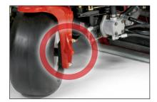
Jack points on all three wheels make removal of front and rear tires a breeze, and fluid sight levels on hydraulic and fuel tanks make daily visual maintenance checks fast and easy.
