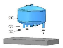
**Step 4** – Attach the extension legs (2) to the media filter legs (7) either using a \*\*quilted forklift or by tilting
