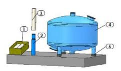
**Step 3** – Place the rubber caps (6) on the bottom of the extension legs (2). \***Note**: The caps fit snugly on only one end of the leg.
