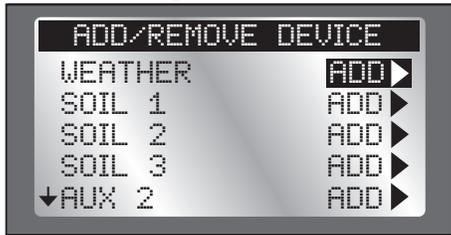
4. The EVOLUTION® controller waits for the identification signal from the weather sensor.
