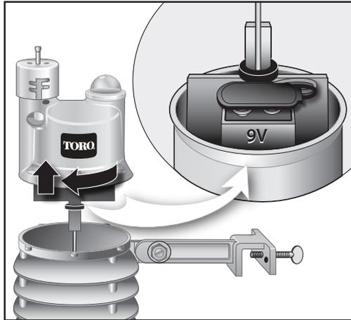
2. Disconnect the battery wire clip. Remove and replace the used battery with a fresh 9V Alkaline battery. Reconnect the battery wire clip.
