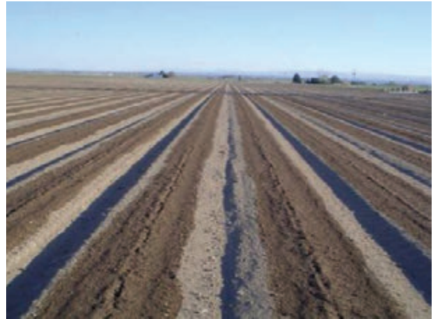
Toro Aqua-Traxx drip tape, 12-inch (30 cm) emitter spacing, .22 gpm/100 ft. (3.09 Lpm/100) on left, 8-inch (20 cm) emitter spacing, .22 gpm/100 ft. (3.09 Lpm/100) on right after 30 hours of irrigation. Note the 12-inch spacing on left has more scalloping.
