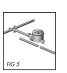
5. To connect the outlet end, cut the poly pipe again, allowing enough gap for the Inline timer unit, and enough poly pipe to connect to the outlet end.
