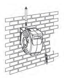
3. Align the back of the reel with the wall bracket and insert the securing pin through the join.
