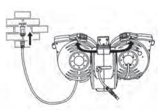
4. Attach the 2m tap to reel connector to your tap using the universal tap adaptor. Test to ensure the reel rotates freely through 180° with the tap adaptor connected.
