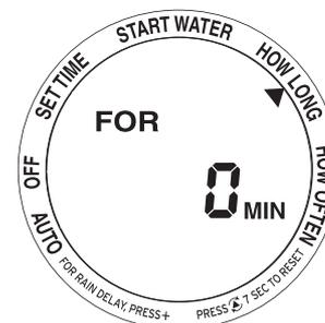
Use the and buttons to set the desired watering duration, up to a maximum of 360 minutes.
