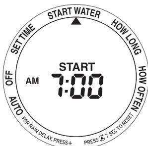
Use the and buttons to set the time that you want watering to start. Press to save the watering start time and go to **HOW LONG** mode.
