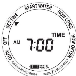
Press to save the time setting and move to **START WATER** mode.
