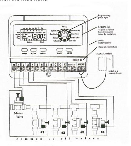
Remove the lower cover. Place the unit on the wall using the top screw slot. Level the controller, and then insert screw into the lower screw hole under the terminal block. Connect the solenoid wires to the terminal block. Connect one wire from the solenoid to its respective station number on the terminal block and the other wire to the C-common terminal. Connect the transformer wires to the 24 VAC terminal.
