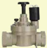
Solenoids act like gates that control the flow of water into your system. A coil magnetises and pulls open a rubber diaphragm letting water pass through. 25mm solenoid valves should be used when considering pop-ups or other systems that require a large amount of water flow.
