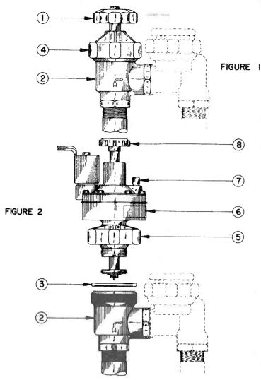
AUTOMATIC VALVE ADAPTER REPAIR KITS L12134 3/4" FITS L2034 L12210 1" FITS L2010
