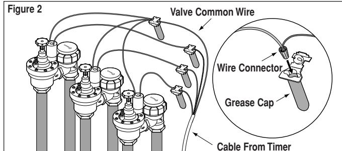
6. Using wire splice connectors, attach either wire from each valve solenoid to the white cable wire. This wire is designated as the valve common wire. Connect the remaining wire from the solenoid to one of the color-coded cable wires. Ensure all wire connections are secure and waterproof.
