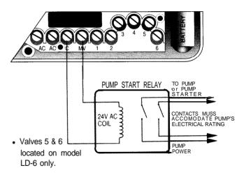
WARNING: If a pump start is installed you must use a jumper wire from each unused terminal screw to a numbered terminal screw in use. This is critical to avoid damaging your pump, (i.e. running it dry, which may burn out the pump motor.) Neglecting to jumper all unused terminal screws may seriously damage your pump during default program execution.
