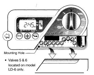
Do not plug transformer into power source until the controller is mounted and ALL valves have been connected.
