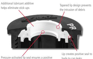
Pressure-activated lip seal ensures a positive seal around the riser and reduces "flow-by"
