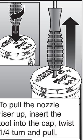
To pull the nozzle riser up, insert the tool into the cap, twist 1/4 turn and pull.
