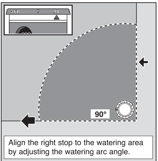
Align the right stop to the watering area by adjusting the watering arc angle.
