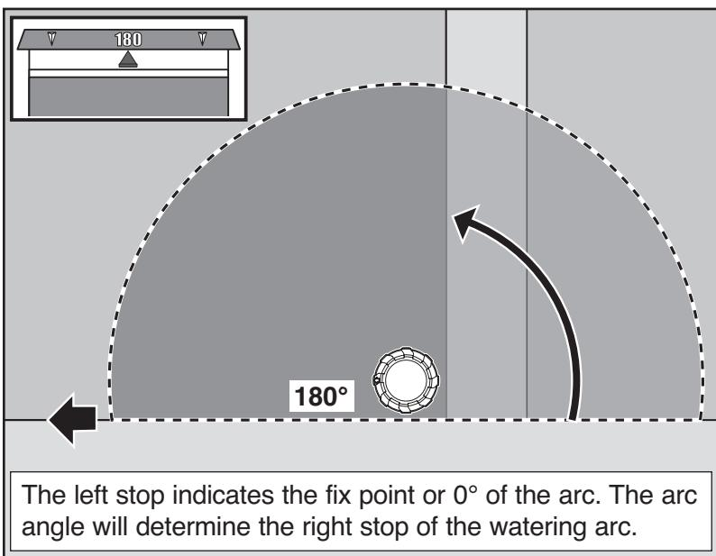
The left stop indicates the fix point or 0° of the arc. The arc angle will determine the right stop of the watering arc.
