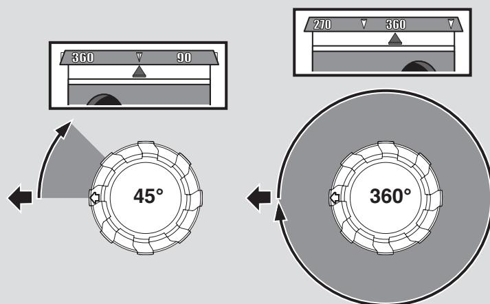
Use the sprinkler tool or a screwdriver to adjust the right stop of the watering arc. Rotate clockwise to increase or counter-clockwise to decrease.
