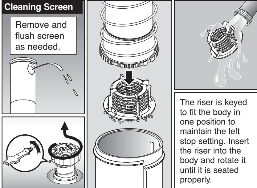
The riser is keyed to fit the body in one position to maintain the left stop setting. Insert the riser into the body and rotate it until it is seated properly.
