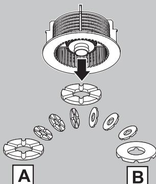
The check valve is factory installed in position A.
