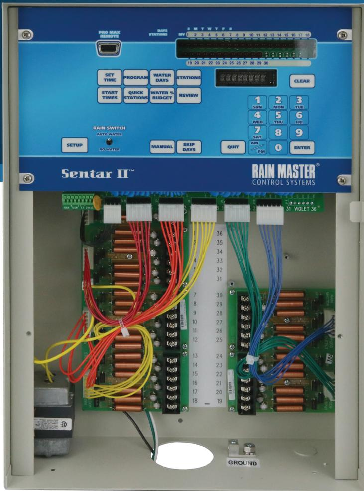
The Sentar II™ has long been noted as the “workhorse” of irrigation controllers. It offers advanced control features for a fraction of the cost of similar models. Designed with the irrigation manager in mind, the Sentar II™ protects landscapes by offering: rain sensing, flow sensing, and cycle and soak scheduling on any of 4 fully independent programs.
