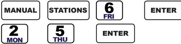
The STATIONS/DAYS display shows the station number 6 and the Master Valve on The PROMPT/MESSAGE display shows the watering time. As time elapses, the displayed watering time will count down. When the controller reaches zero, the station shuts off and the controller will return to the Automatic Mode.
