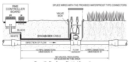
Figure 10 - Flow Sensor Electrical Connections
