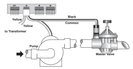
Figure 6 - Master Valve and Pump Electrical Connections
