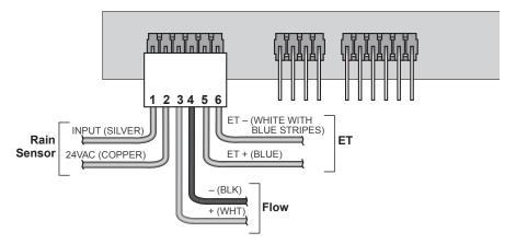
Figure 11 - Sensor Interface Electrical Connections
