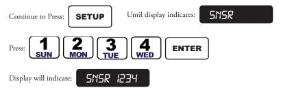
The Rain Master Eagle is now configured to use a Rain Sensor for all programs. The controller will automatically shut off irrigation if a rain storm occurs and will automatically restart irrigation after the rain storm has passed and the rain sensor has dried out.
