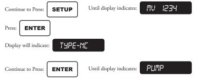
The Rain Master Eagle is now configured to use a Normally Closed Master Valve for all programs. The Master Valve will open when any irrigation program runs.
