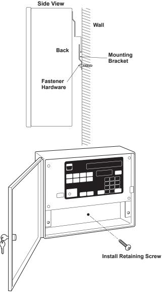
Figure 3 - Controller Mounting
