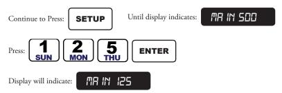
The Unscheduled Flow Limit is the maximum flow that the Rain Master Eagle will allow whenever the Rain Master Eagle controller is not in use. This feature is used when a Normally Open Master Valve has been installed and you wish to have a small amount of water available for manual use.
