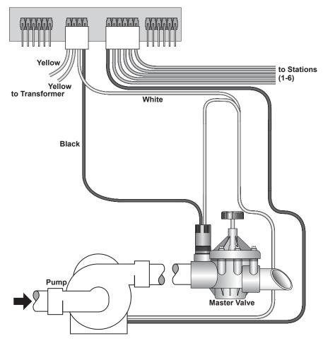
Figure 9 - Normally Open Master Valve and Pump
