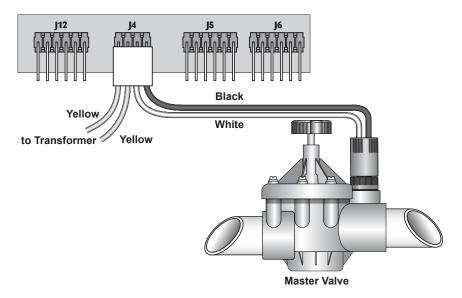
Figure 5 - Master Valve Electrical Connection
