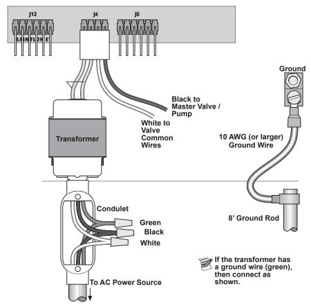
Figure 4 - Power and Grounding Connections
