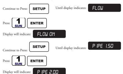
The Flow Sensor has been enabled for a pipe size of 2 inches and is applicable to all irrigation programs.
