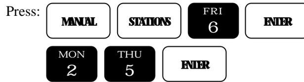
The display will indicate the station that is running and the associated watering time. As time elapses, the watering time will display the watering time remaining. At completion of the watering time, the station will shut off and the controller will return to the Automatic Mode.
