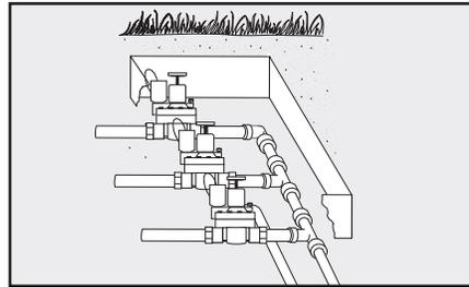
These valves are primarily used with wells, or where codes require a separate backflow-prevention device. They're usually installed below ground and protected by a valve box.
