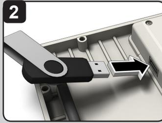
2 Insert USB drive into the controller USB slot.
