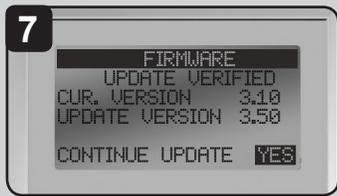
7 Controller displays the firmware version in the controller (*current*) and the version on the USB drive (*update*).
