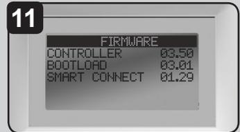
11 Go to ADVANCED-->FIRMWARE-->VERSION and confirm the firmware has been updated to 3.50 and bootload version 3.01. The update is complete.
