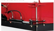
The hydraulic relief feature of the 180Z actively protects the wings and blades when in contact with an obstacle-in either forward or reverse.
