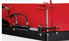
The hydraulic relief feature of the 180Z actively protects the wings and blades when in contact with an obstacle - in either forward or reverse.
